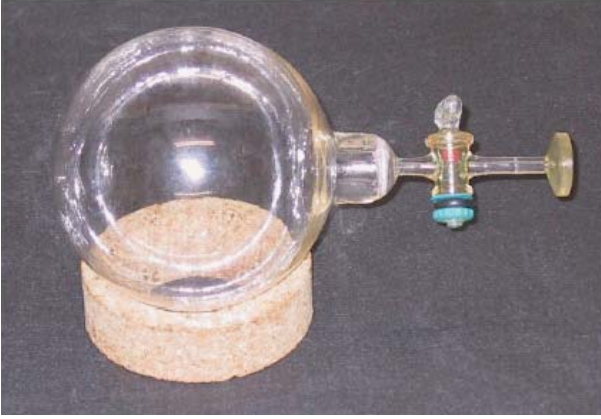
Fig. 4. Photograph of a 1.1 litre storage- and transport cell made from iron-free Corning 1720 glass produced on special demand by Schott AG Mainz.
